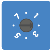
Rotary switch set to position 2
