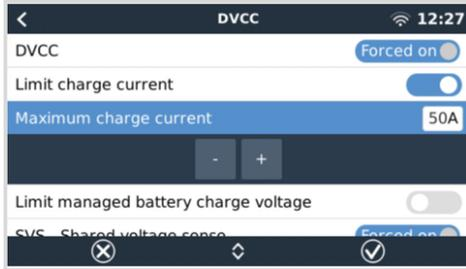
Limit charge current is a user-configurable maximum charge current setting. It works across the whole system. MPPT solar chargers are automatically prioritised over the mains/generator.
