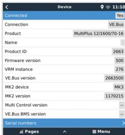
The Device menu (Device List → [Multi or Quattro] → Device) offers device-related parameters such as custom name setting, firmware version, serial numbers (in the sub-menu) and more that can be used for diagnostic.
