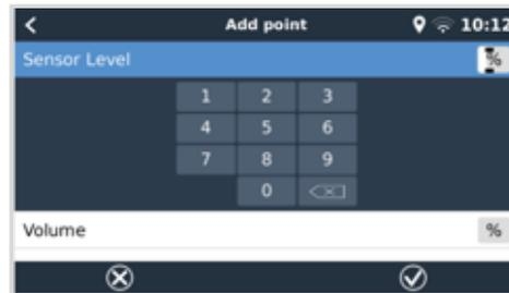
The tank level ports can each be configured to work with either European (0 - 180 Ohm); or US tank senders (240 - 30 Ohm) standards; or to configure a custom Ohm resistance range between 0 Ohm and 300 Ohm (requires firmware v2.80 or higher).
