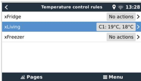
In GX products where two relays are available (Cerbo GX & Cerbo-S GX, Ekran GX), it is possible to have a single temperature sensor control both relays. It is also possible to have a single relay controlled by multiple different temperature sensors. For example, a Cerbo GX with 2 lithium battery heat pads, and only using both simultaneously when necessary.
