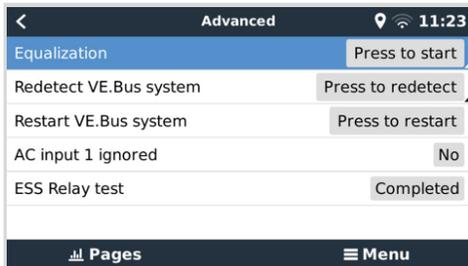
The Advanced menu can be accessed from Device List → [Multi or Quattro] → Advanced and contains options for equalisation, redetect and restart VE.Bus system and shows the ESS relay test status.
