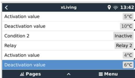
This will mean that Relay 1 will be active if the battery temperature falls to 5 degrees. If the temperature continues to fall below 5 degrees to 4 degrees, then the second heat pad will be engaged via Relay 2. If that is sufficient to raise the temperature back to 6 degrees, Relay 2 will deactivate, and then Relay 1 will remain active until battery temperature returns to 10 degrees.
