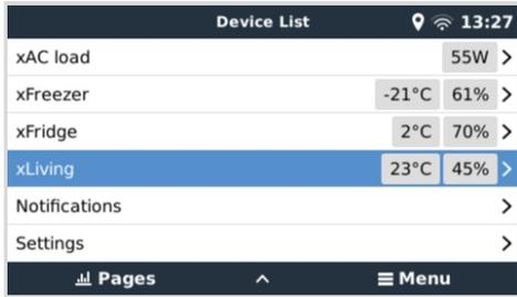
The temperature relay is controlled from Settings Menu → Relay → Function (Relay 1/2) → Temperature. Once enabled, the Temperature control rules menu will appear in the Relay menu, and inside the temperature sensors that have been detected.
