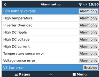
When using a VE.Bus system, it is possible to configure the severity of problems on the VE.Bus system that should cause a notification to show up on the Cerbo GX (and make it beep).
