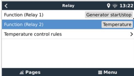
Each temperature sensor can be used to control the relay. Select the temperature sensor you wish to use to control the relay. The temperature sensors that aren't used will display "No actions". It is possible to enable or disable the temperature relay control for each temperature sensor within this menu.
