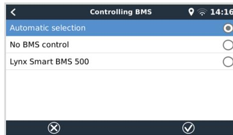
For systems with multiple BMSs connected, this allows selection of which BMS to use for DVCC. This also allows the use of a BMV or SmartShunt for SoC tracking by selecting a BMV as battery monitor (Settings → System setup) while the BMS is still used for DVCC.
