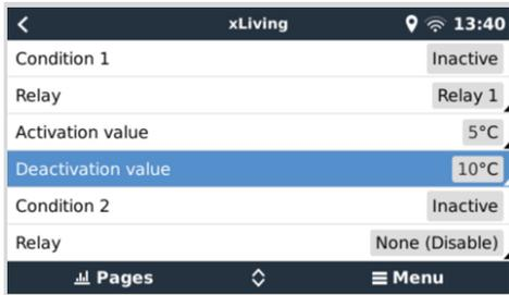
If that is insufficient to maintain the battery temperature above 5 degrees, you may wish to connect a second heat pad contactor to Relay 2 as well.
