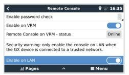
The Remote Console menu (Settings  $\rightarrow$  Remote Console) contains options for controlling access to the Remote Console via LAN/WiFi and VRM and shows the online status of the Remote Console on VRM.
