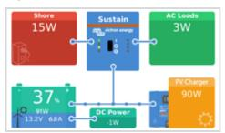
The solar and wind priority function ensures that solar and wind energy are used to charge the battery. At the same time, shore power is only used to prevent the battery from becoming too deeply discharged.
