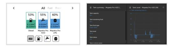
Tank levels can be monitored at various locations within the GX environment:
