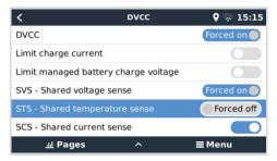
Select the temperature sensor to use; and the GX device will send the measured battery temperature to the inverter/charger system as well as all connected solar chargers.
