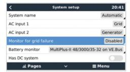
When this feature is enabled, an alarm is raised when the system hasn't been connected to the AC input configured to be Grid or Shore for more than 5 seconds.
