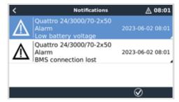
This alarm is triggered once the inverter/charger has received CVL/CCL or DCL data from a managed battery and will shut down if the battery is disconnected or communication with the battery get lost. The alarm is also raised when the inverter/charger has lost connection to a VE.Bus BMS.
