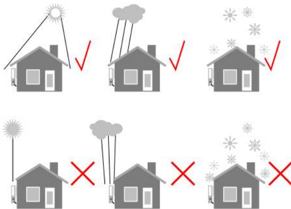
Figure 14 Inverter exposure requirements
