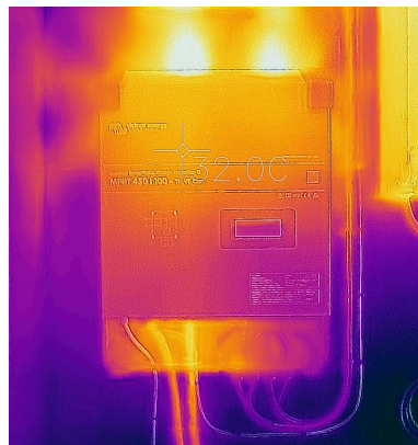
Figure 1. Thermal image of MPPT RS heat zones required for clearance.
