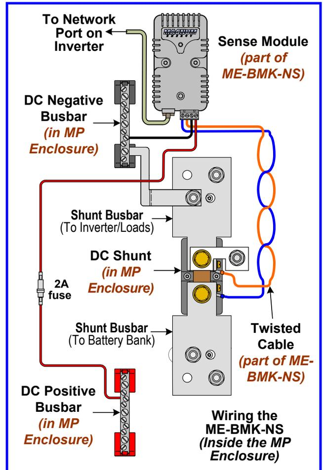
**Figure A2-1, Accessing the DC Shunt**
