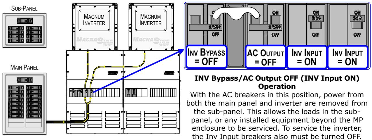
**Figure 5-3, 125A Bypass Switch Operation (MPSH-30D and MPDH-30D)**
