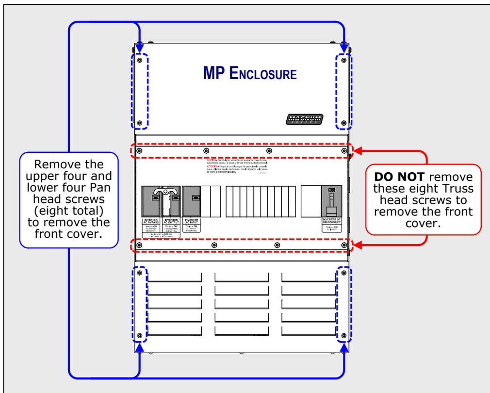
**Figure 3-7, Front Cover Screws to Remove**
