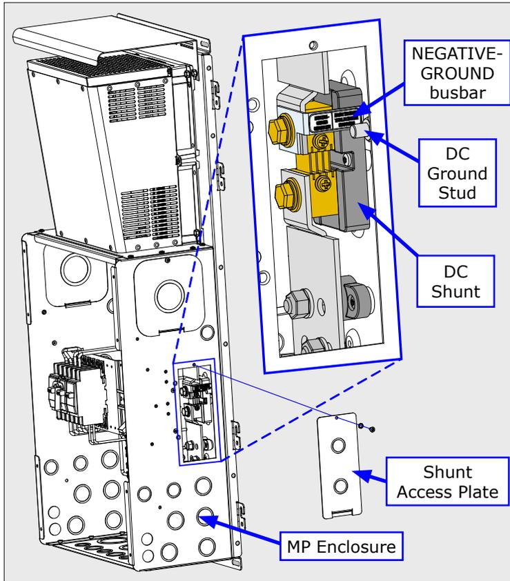
Follow the steps below to remove the NEGATIVE-GROUND busbar (refer to the diagram to the left to help locate the components discussed):
