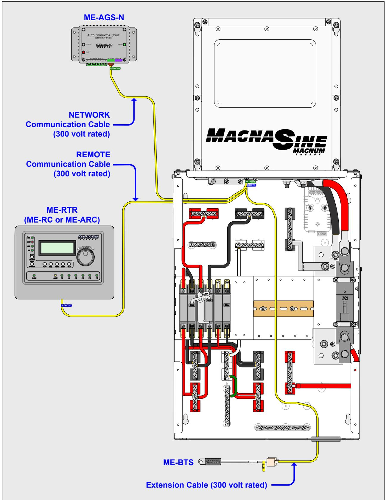
**Figure 3-27, Accessory Wiring Using 300 Volt Communications Cables**
