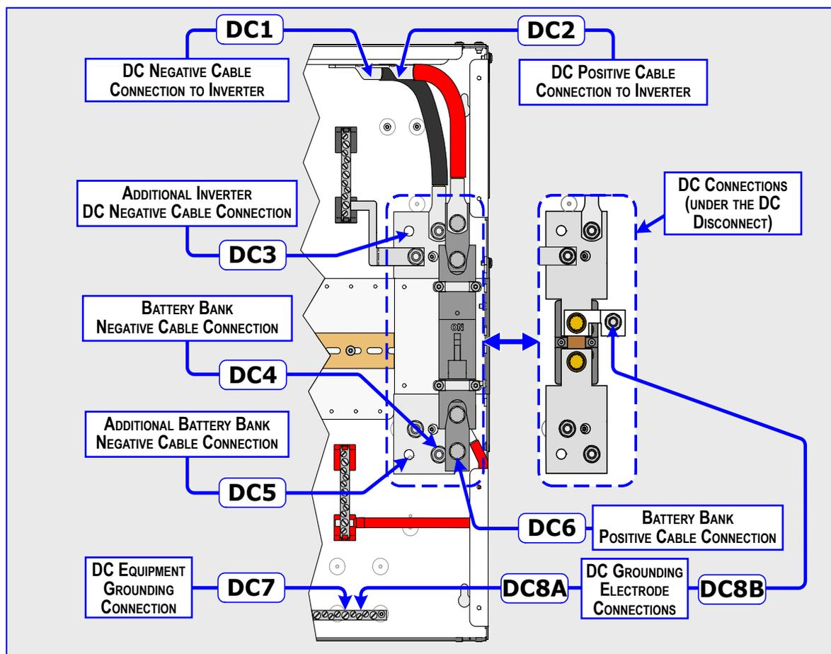
**Figure 3-21, DC Wiring Connection Points for MPSL Models**
