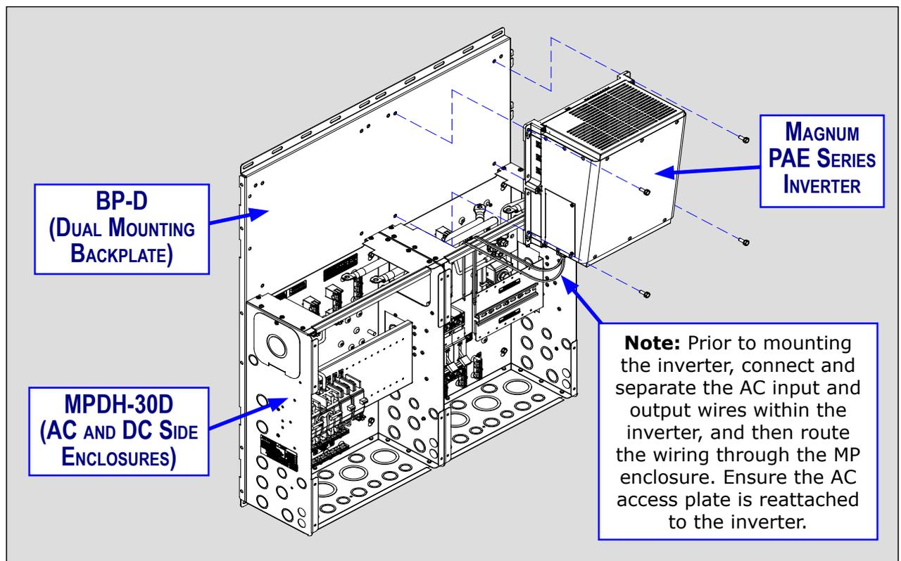
**Figure 3-16d, Mounting First Inverter - MP Dual Enclosure**
