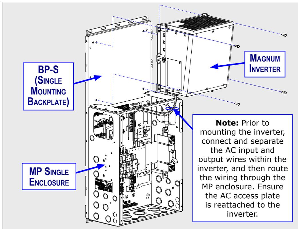
**Figure 3-15b, Mounting Inverter - MP Single Enclosure**
