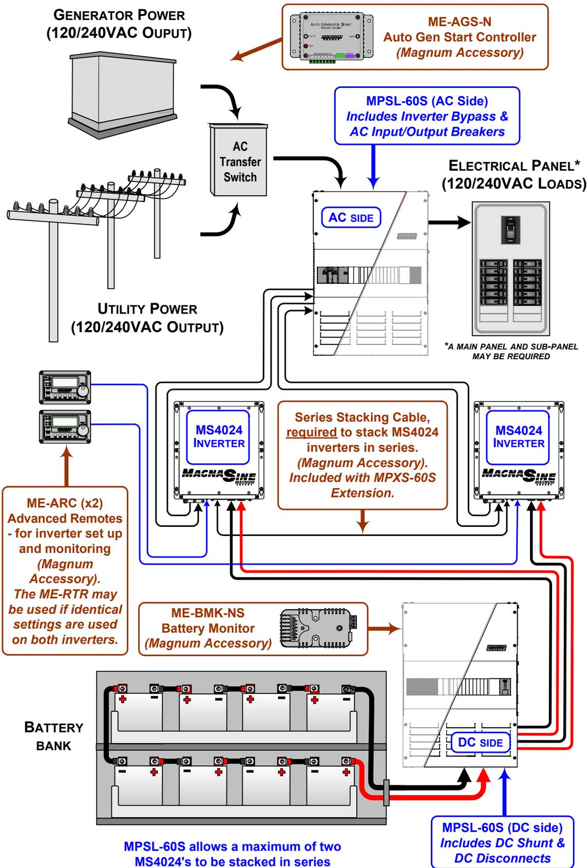
**Figure 3-4, MP Series Simplified Series-Stacked Installation Diagram**
