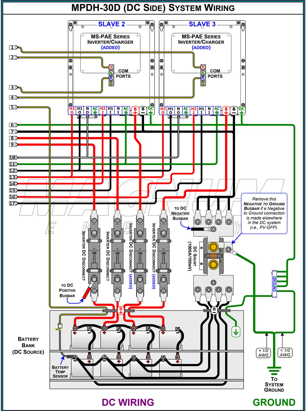
Figure 4-6f.2, MPDH-30D Full System Wiring Diagram (DC Side)
