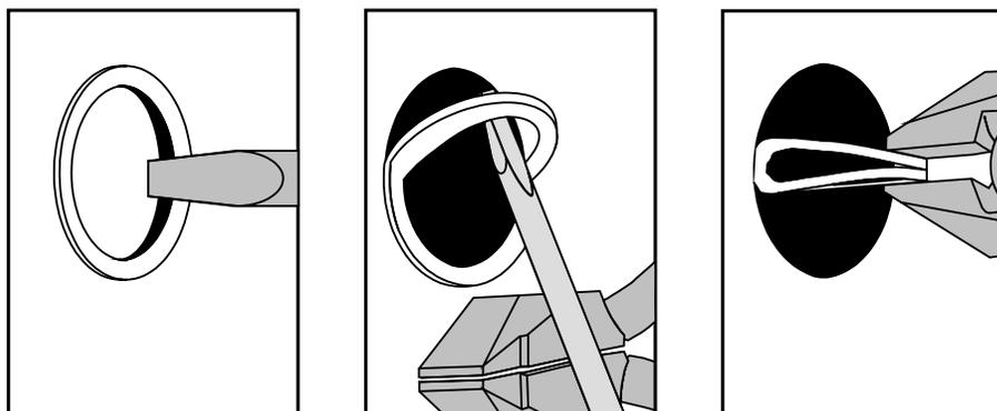
**Figure 3-11, Removing Knockouts**
