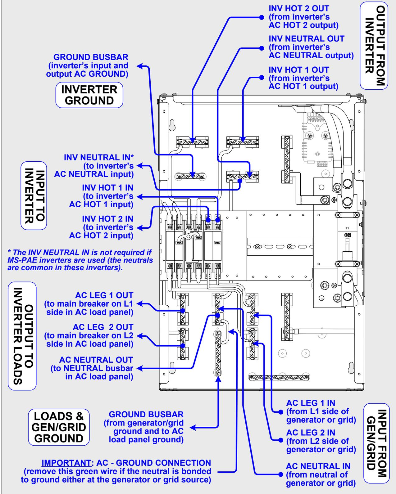
Figure 3-17, MPSL-30D and MPSH-30D AC Wiring Connections
