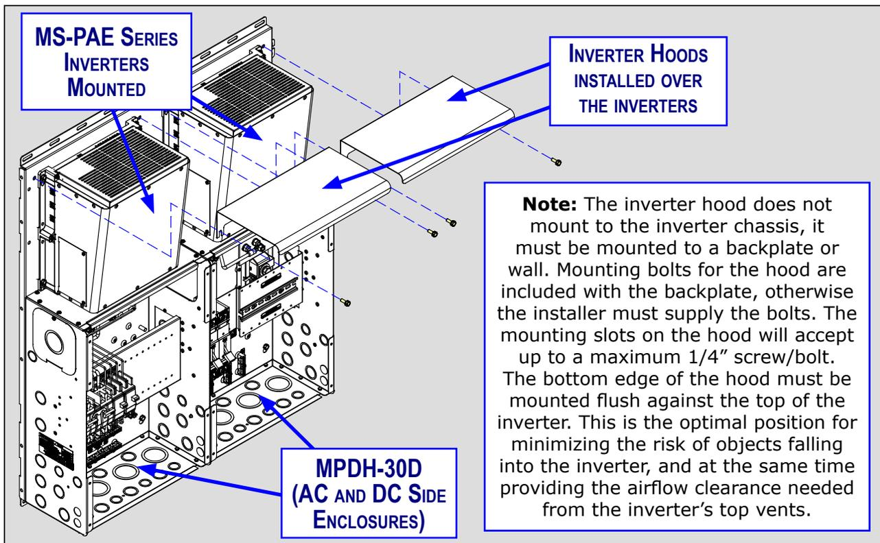
**Figure 3-16f, Mounting the Inverter Hoods - MP Dual Enclosure**
