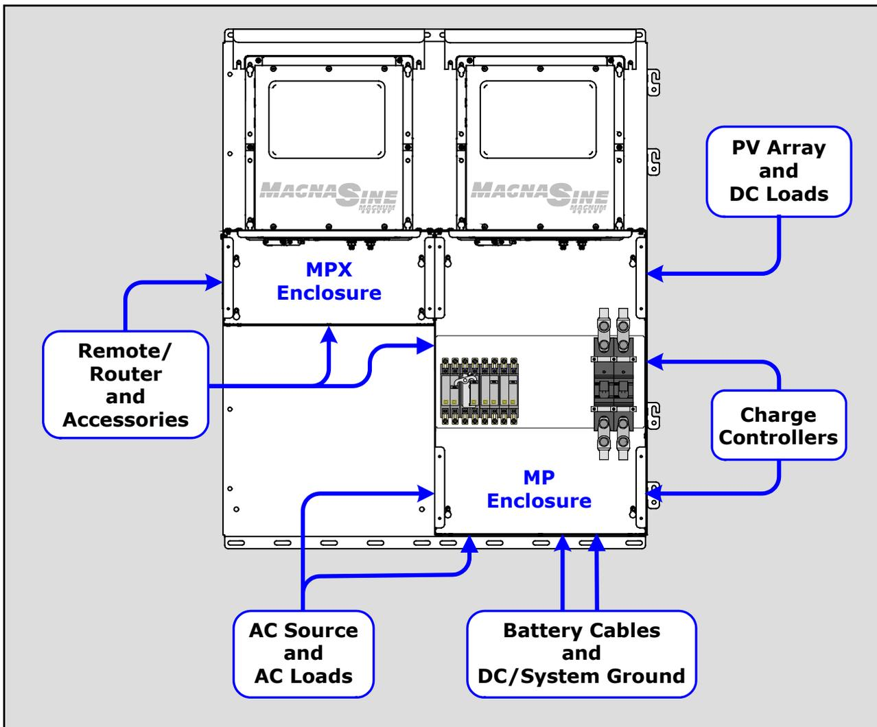
**Figure 3-10, Conduit/Wire Routing**
