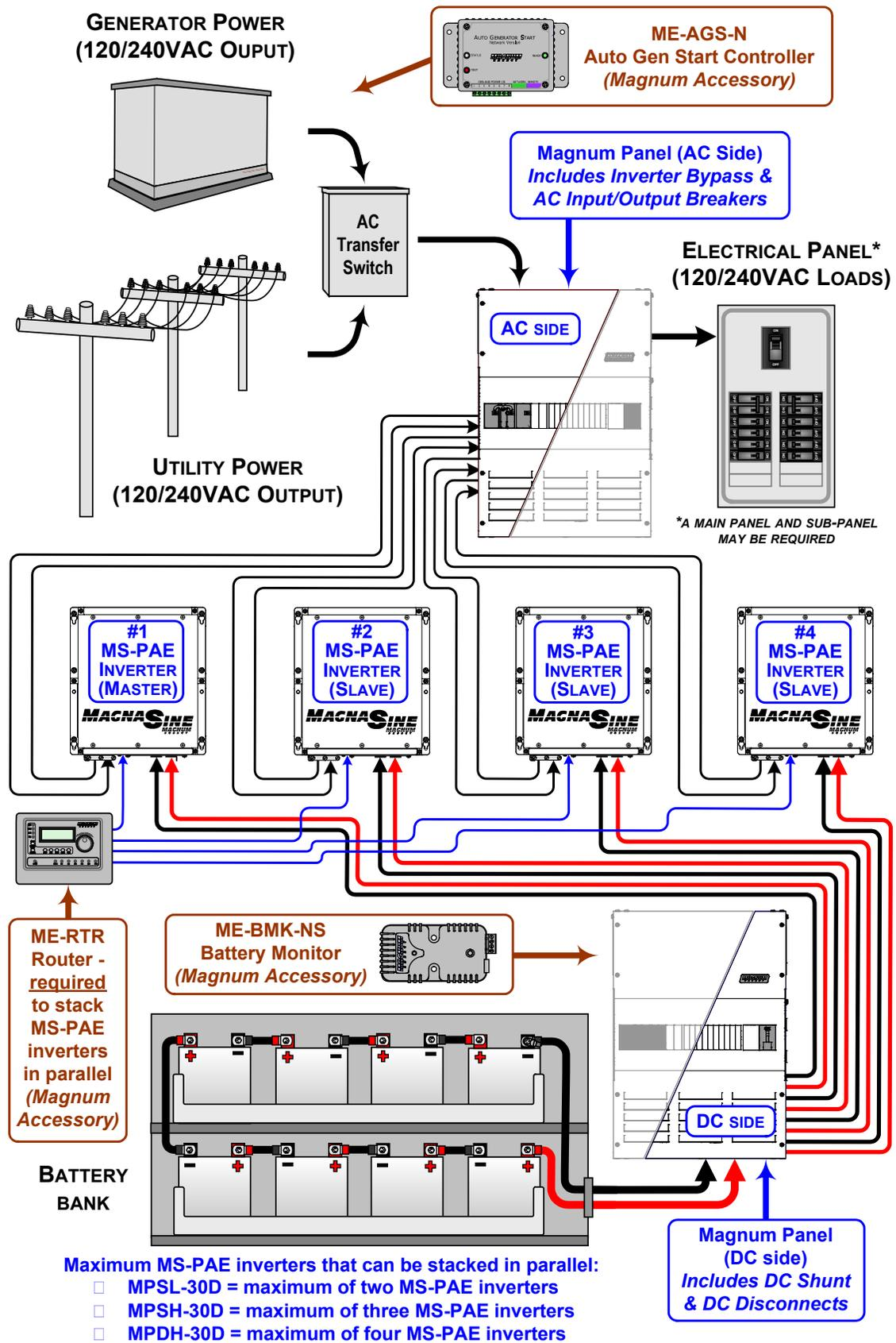
Figure 3-3, MP Series Simplified Parallel-Stacked Installation Diagram
