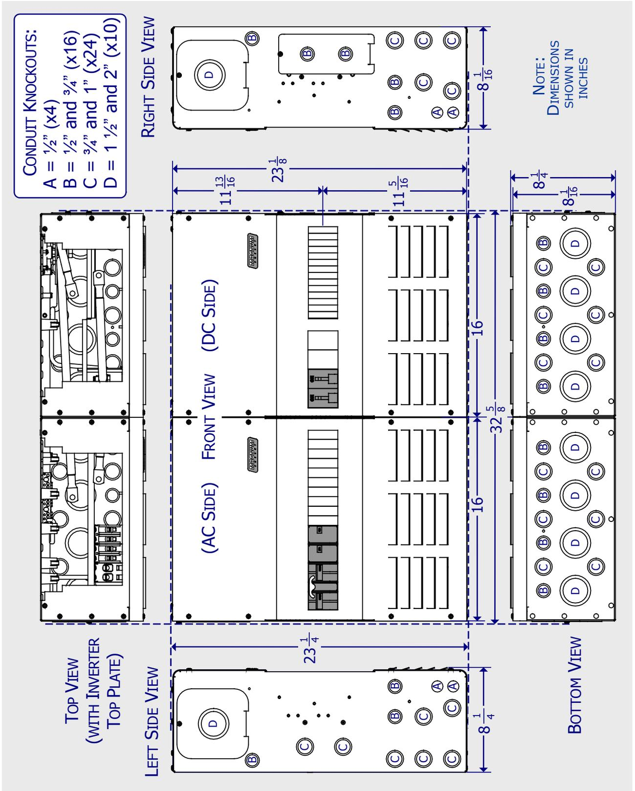
Figure 3-14, MPDH Dimensions and Knockout Location/Sizes
