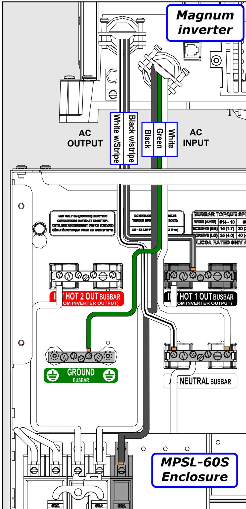
**Note:** This figure shows wiring inside the MPSL-60S for one MS4024 - as LEG 1 (120V AC only). A second MS4024 can be connected in a Series-stacked configuration - as LEG 2 (120/240V AC). Refer to information on the MPX Extension models for stacking a second MS4024 in series.
