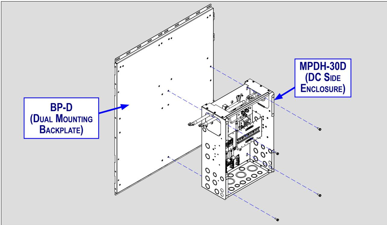
**Figure 3-16a, Mounting the MP Dual Enclosure (DC Side)**
