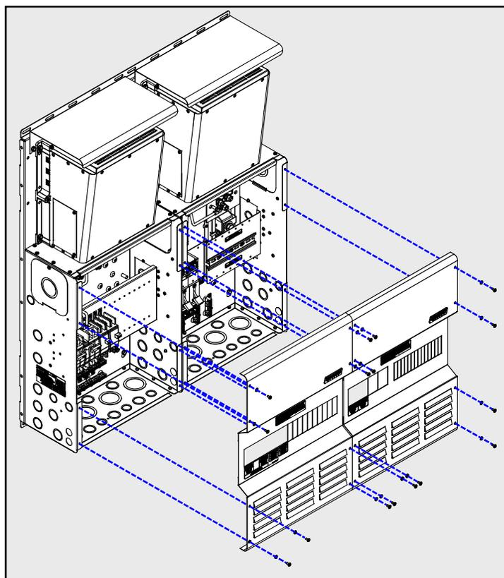
**Figure 3-40, Attaching Front Covers - MP DH Models**
