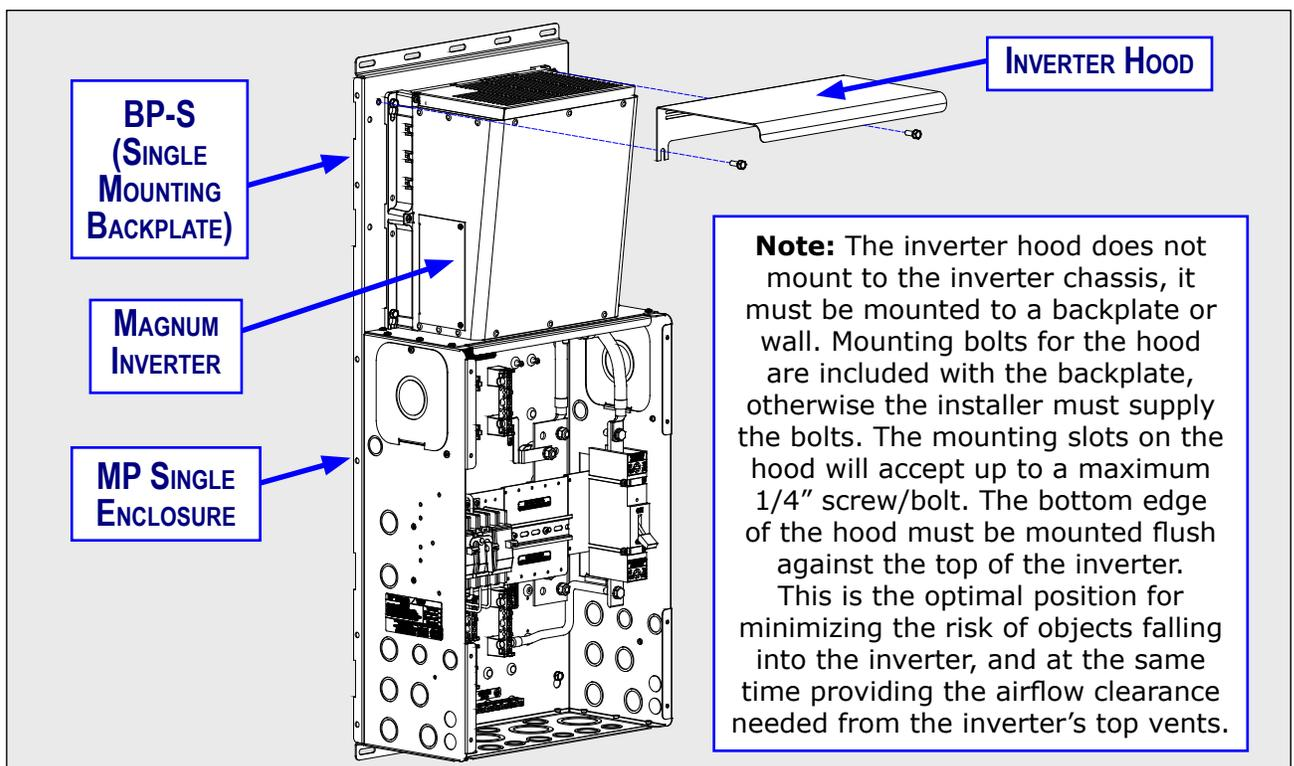
**Figure 3-15c, Mounting Inverter Hood - MP Single Enclosure**
