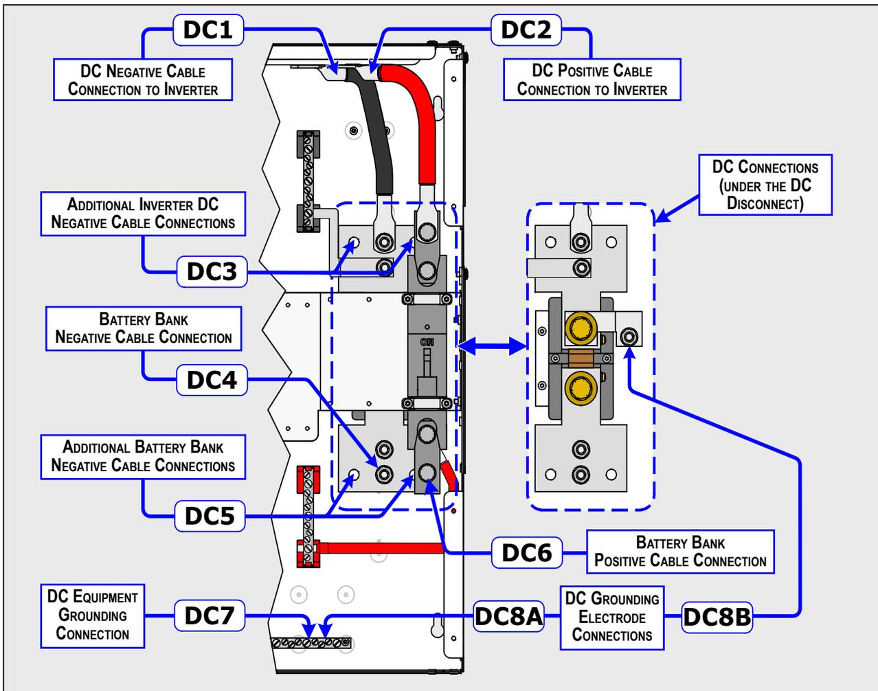
**Figure 3-22, DC Wiring Connection Points for MPSH-30D**
