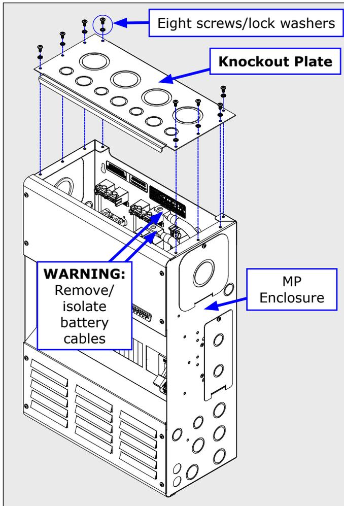
Figure A5-1, Attaching Knockout Plate
