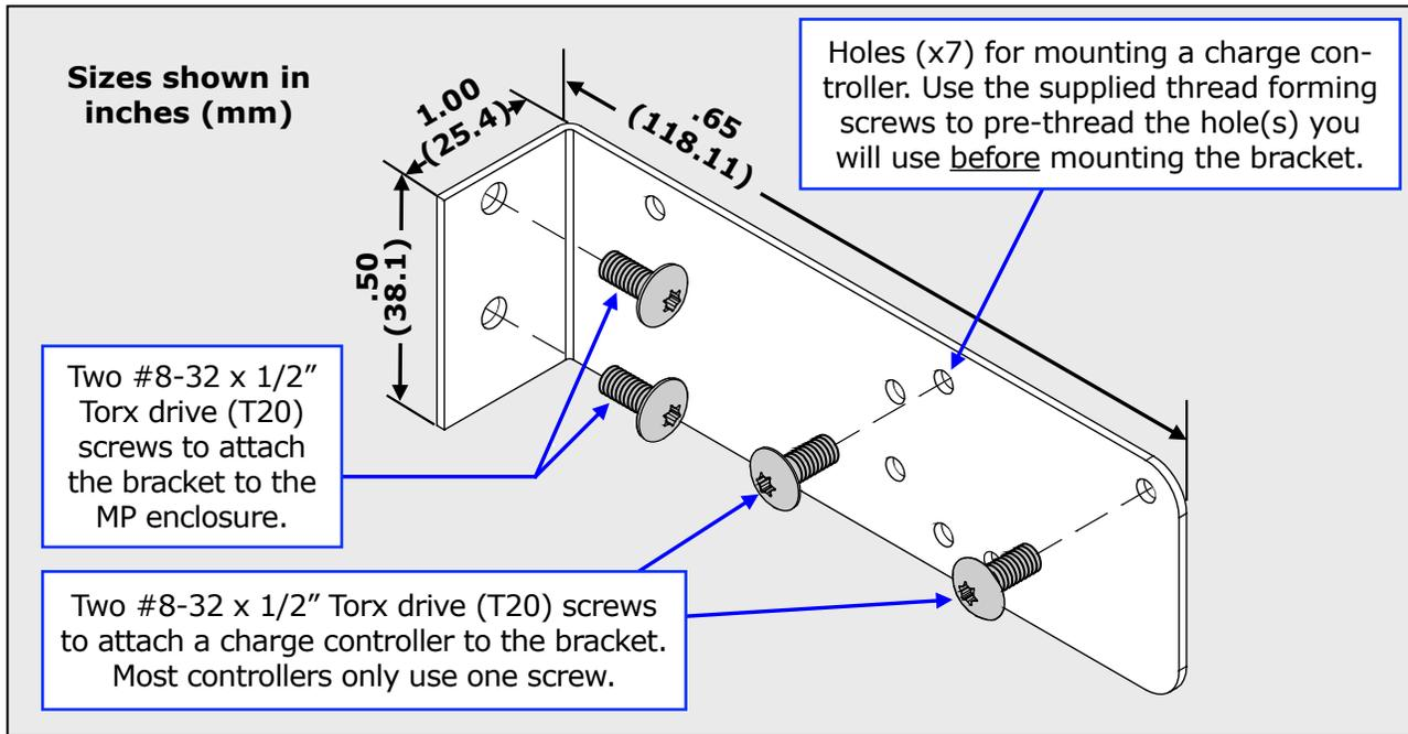
**Figure A1-1, Charge Controller Bracket - Physical Dimensions**
