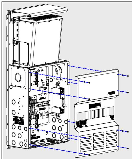
**Figure 3-39, Attaching Front Cover - MP SL/MP SH Models**
