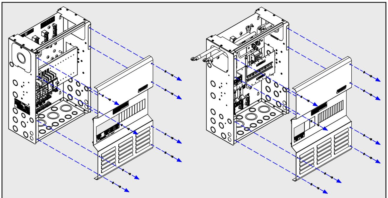
**Figure 3-9, Removing Front Covers - Dual Enclosure**
