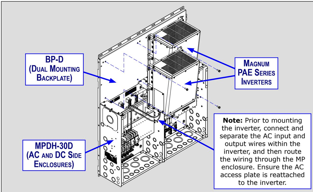
**Figure 3-16e, Mounting Second Inverter - MP Dual Enclosure**
