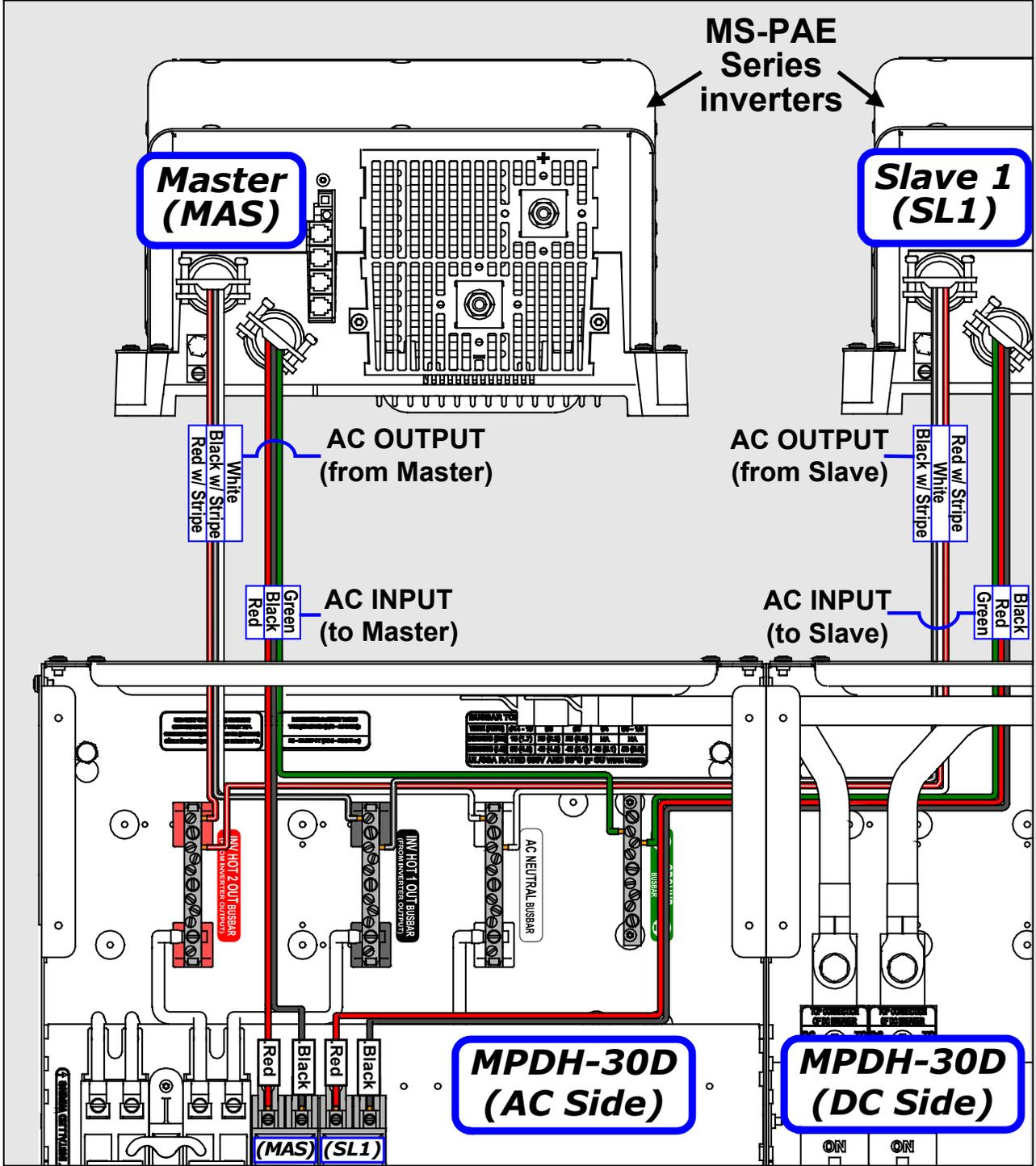
Figure 4-6a, MPDH-30D Inverter AC Wiring
